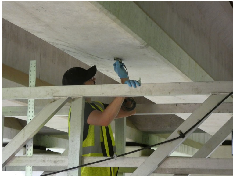
(a) Attaching BDI Reusable Strain Gages
